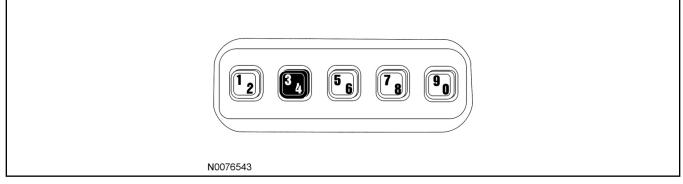
3. To unlock the trunk or hatch, if equipped, press the 5/6 button within five seconds of entering a valid keypad code (IKT vehicles may require the 5/6 button to be pressed twice). Press the 5/6 button twice to open or close the passenger side power sliding door, if equipped.
