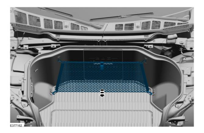
4. Remove the load compartment floor storage cover.
