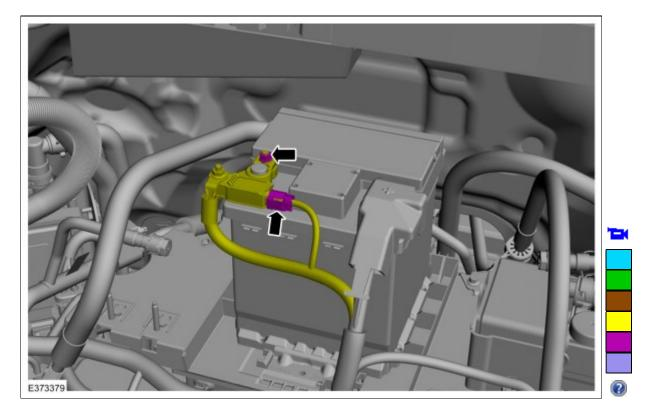
5. Position the positive battery cable terminal cover aside.
