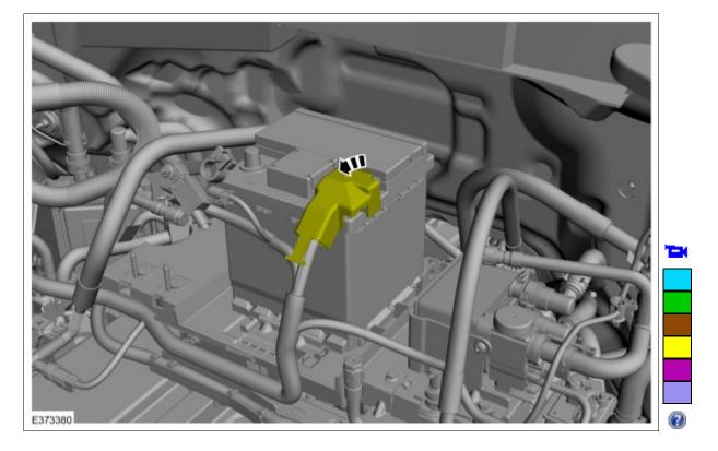
6. Loosen, but do not remove the nut and position the positive battery cable aside. *Torque*: 55 lb.in (6.2 Nm)
