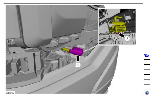
8. Disconnect the active grille shutter actuator electrical connector.
